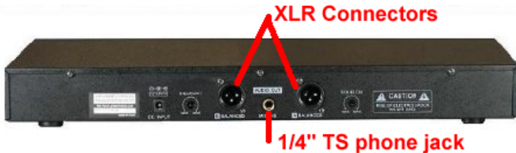
Figure 2 – back of GTD Audio 622 showing XLR connectors and 1/4" phone jack
